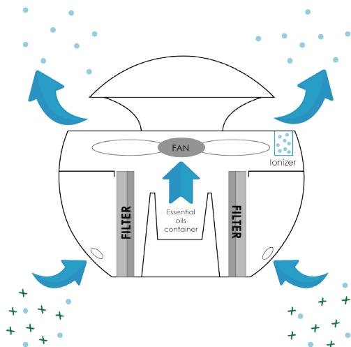
The fan sucks the air through the openings situated under the appliance. The air is purified thanks to an E11 type particle filter which retains pollens, bacteria and small particles.
